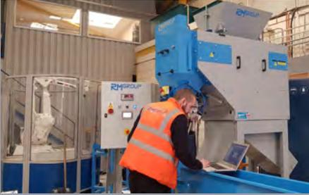
Developed in response to the need for a simple “operator” friendly interface platform, RMGroup software engineers extract the commonly required process controls from the complex robot programming pendant and make them available on a simple to use and understand touch screen display.
