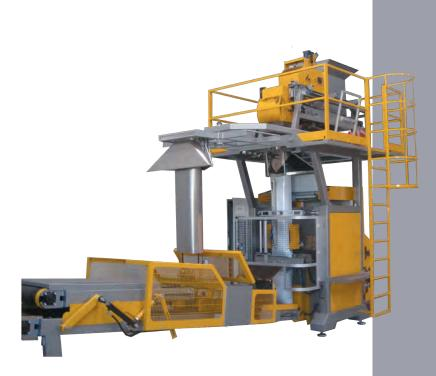
The FPK 50 lends itself to bulky products. However an advantage of using the FPK 50 is that it is capable of bagging in smaller bag sizes. This system is also suitable to those looking to use a euro pallet for bigger bags.
