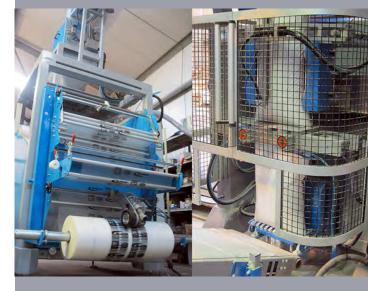
The FPK 48 follows the FPK 46 in the Form, Fill and Seal range. It has a larger film reel width for production of larger bag sizes. Previous applications used with this machine include coal, animal feeds and wood pellets.
