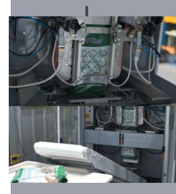
The FPK 44 is one of the most popular Form Fill & Seal vertical bagging systems. It proves to be extremely versatile to handle most applications. Previous installations include packaging lines for wood pellets, animal feeds, rock salt, wet sand and other aggregates.
